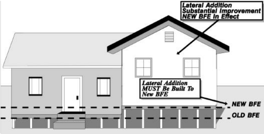
Figure 8-9. Substantial improvements to post-FIRM buildings must be elevated above the new BFE. Nonresidential buildings may be floodproofed
